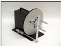
The MINI-CATs have an inner label flange to keep the edge of the label web aligned as the labels are being rewound. Also available is an optional Adjustable Paper Guide (**APG-MC**) that mounts directly to the **MC-10** or **MC-11** base plate and guides the outer edge of the labels. For the **MC-10**, an optional plastic Outer Flange (**2<sup>nd</sup> Flange MC-10**) is also available.
